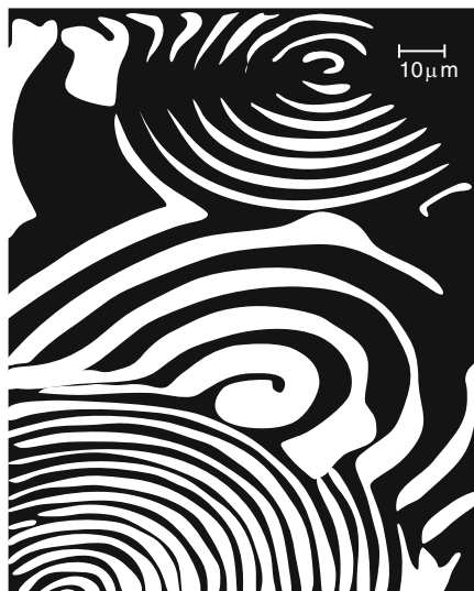
Fig. 8.13. Photoemission electron microscopy (PEEM) image of a Pt(110) surface exposed to 4 \times 10^{-4} mbar \text{O}_2 and 4.3 \times 10^{-5} mbar CO at a temperature of T = 448 K. (After [479])
